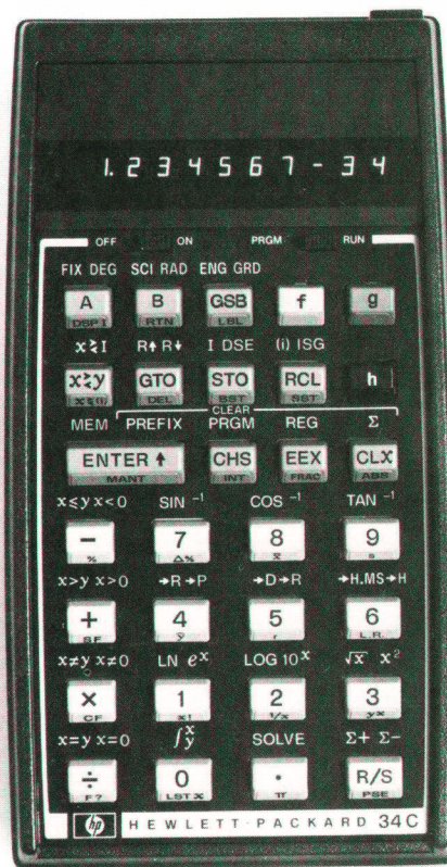
Fig. 1. The HP-34C, a new handheld programmable calculator, has two keys that are new to handheld calculators— \int (integrate) and SOLVE SOLVE , a numerical equation solver, is described in this article.
